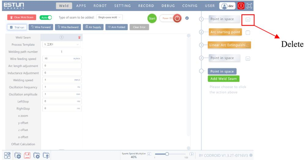
According to the actual working conditions, the motion instructions can be customized, and the programming of combination welds such as straight line, straight line plus circular can be realized.
