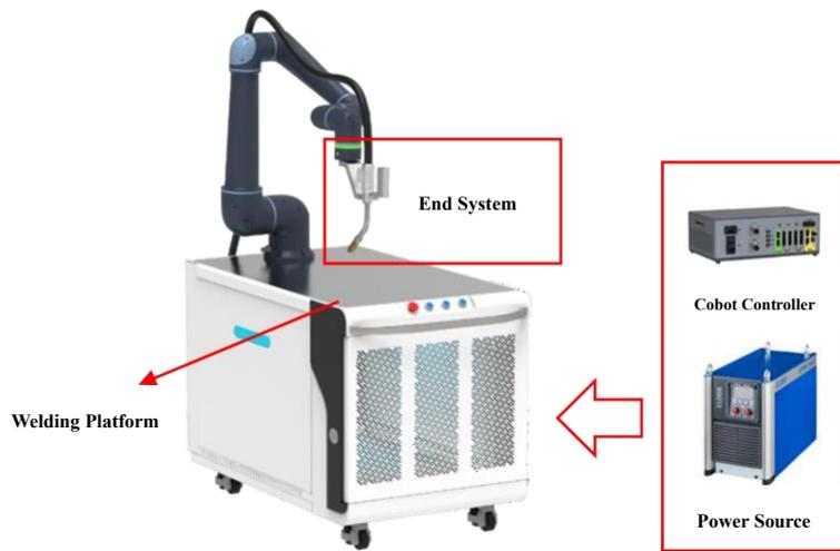
Pic 3-1a Welding Workstation (Arc Welding)
