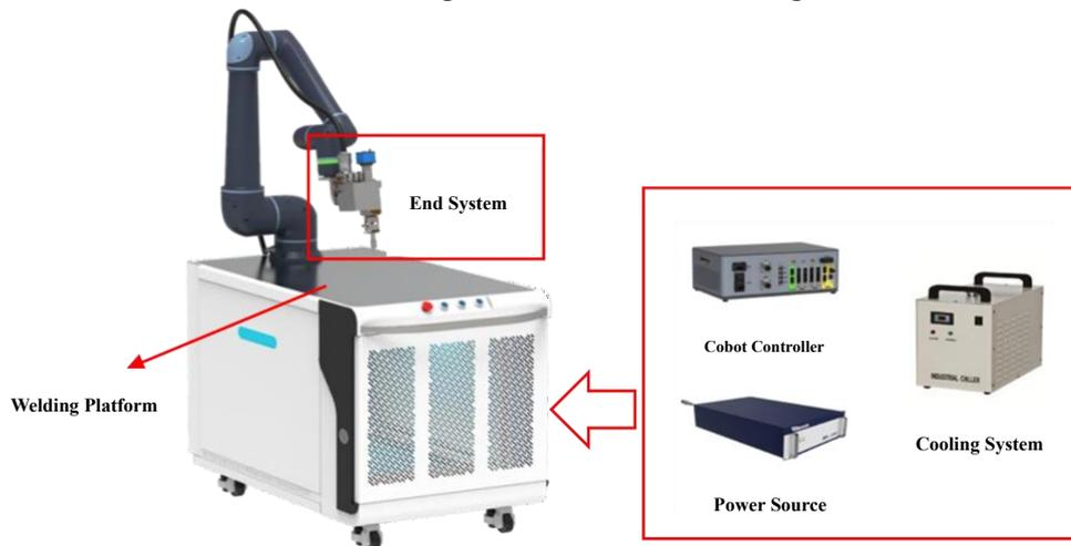
Pic 3-1b Welding Workstation (Laser Welding)
