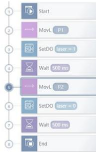
2. Move to welding start point (P1) by linear motion
