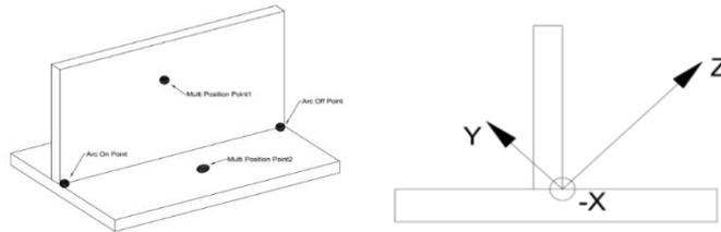
Note: The reference points must be on both sides of the teaching weld. TCP as close as possible to the location you want to teach; The welding direction must be consistent.
