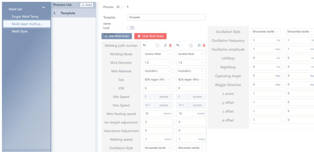
As shown in the figure above, each parameter in the multi-pass can be set independently, among which X scaling, Y offset, Z offset and a offset are unique parameters of the multi-pass and are set to offset the base pass. The specific setting method is as follows.
