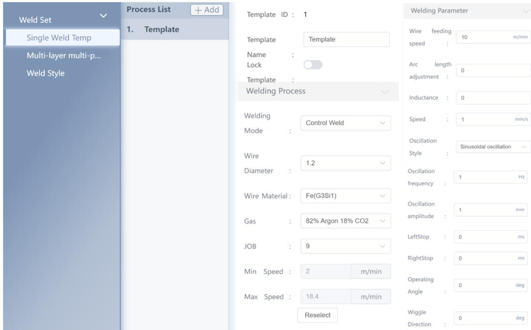
Welding Process-Wire Material<sup>①</sup>: Select the welding wire material in the process curve of CLOOS welding machine, respectively: AlMg2,7Mn, AlMg4,5Mn, AlMg5, AlSi5, CrNi 1.4316, CrNi 1.4370, CrNi 1.4462, Fe(G3Si1), Fe-basis, Fe-Met, Fe-RUT.
