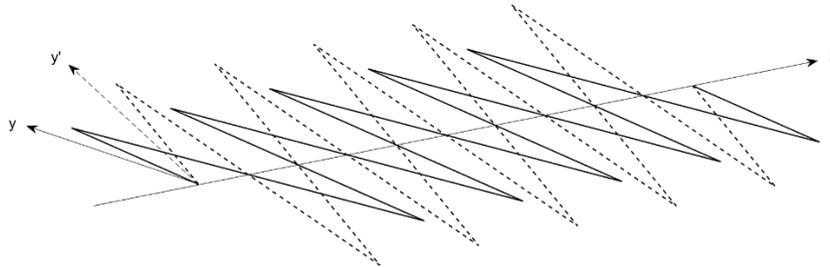
**Weaving Direction:** The tilt of the weaving direction in the weaving plane can be adjusted. The weaving direction cannot be negative, and the legend is 10° weaving direction.
