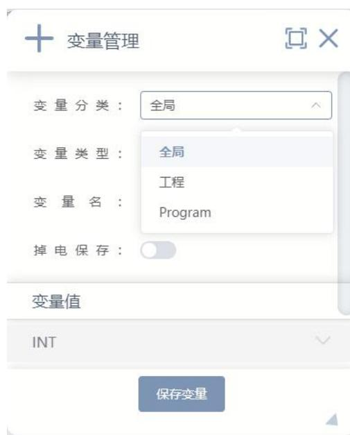
In the variable label button, you can click to add a new variable, select a different variable classification, type to add the selected variable classification, type, specific
