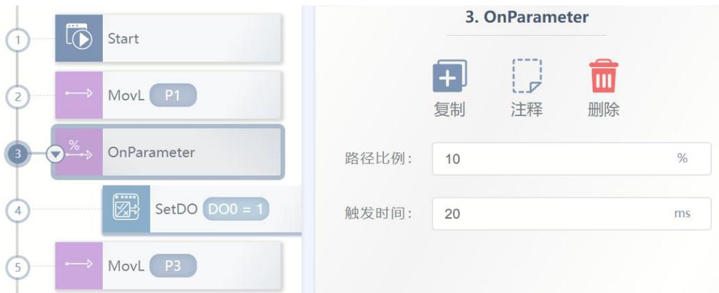
The legend indicates that when the robot TCP moves from P1 to P3, DO0 is set to 1 20ms in advance when it moves to 10% position. If the trigger time is changed from 20ms to -20ms, it means that the DO0 is set to 1 when the robot moves to 10% position 20ms in advance.
