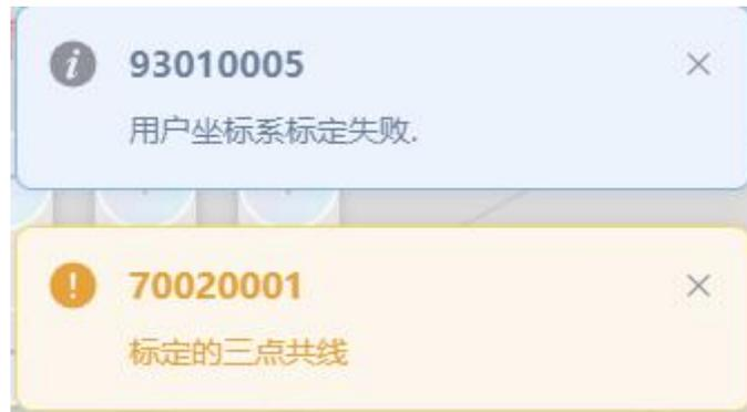
If the "Calibrate USERCOOR" window does not automatically fill in any values and is accompanied by a "user coordinate calibration failed" message, the calibration failed.
