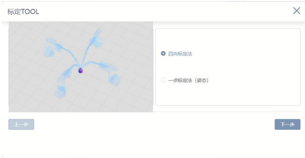
Move the robot (click or drag) to four different positions, each time touching the tool point with the same needle tip placed in the space and clicking the "Direction Show" button. The four positions are performed to obtain the TCP translation relationship with respect to the center of the tool output flange.
