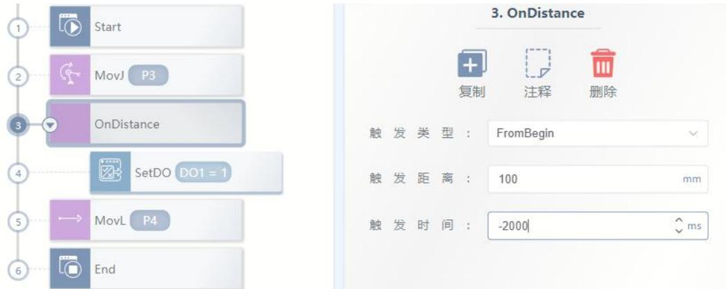
The legend indicates that when the robot TCP moves from P3 to P4, DO1 is set to 1 2000ms before moving to the position of 100mm. If the trigger time is changed from -2000ms to 2000ms, it means that DO1 is set to 1 2s after the robot moves to the 100mm position.
