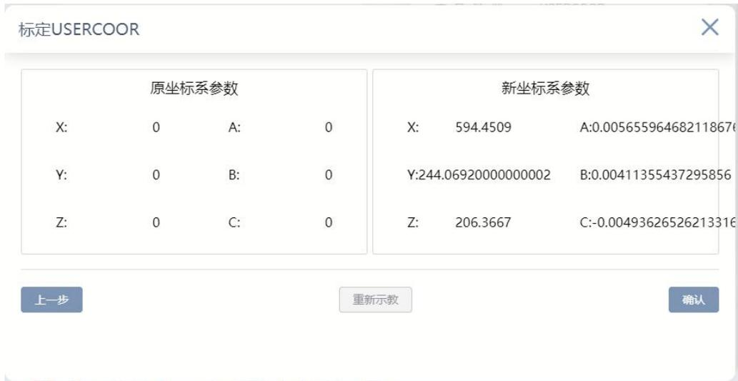
The values of x,y and z of the user coordinate system will be automatically filled into the "Calibration USERCOOR" window, click the button to complete the calibration guide, and then choose whether to save the variable. 确认
