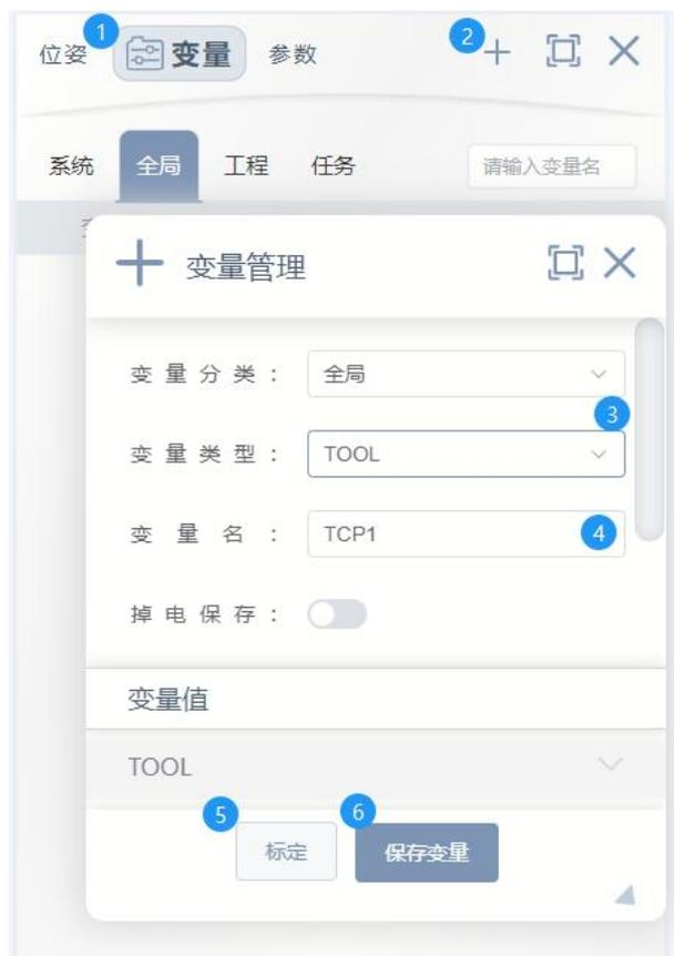
When the tool coordinate system needs **to be calibrated**, the **"four-way calibration method"** and **"one-point calibration method (attitude)"** can be used to obtain the translation and rotation of TCP (tool center point) relative to the center of the tool output flange.
