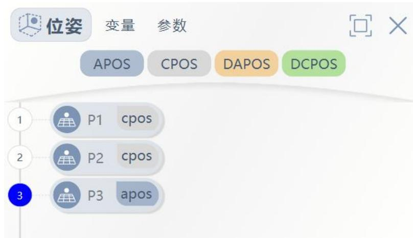
Double-click on the Pose TAB button to add a new pose. Select a different pose type to add the selected pose. Four pose types are:
