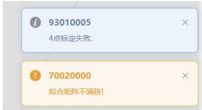
If the Calibration TOOL window does not automatically fill in any values and is accompanied by a "4-point calibration failure" prompt, the calibration failed.
